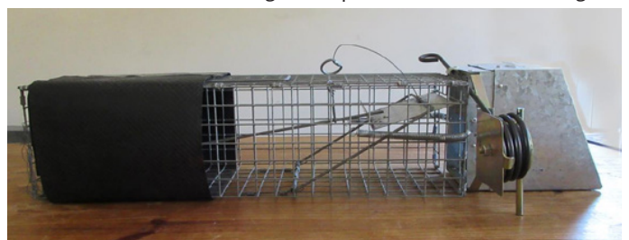
Figure 12 A few minor alterations to the Kania 200 spring trap housing allow it to be fitted tightly to the entrance of a live capture trap. The back of the housing can also be cut out and a perspex window inserted to encourage the squirrel to run toward the light.
